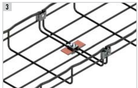
3 Add another SWK to the bottom section over the copper strips for proper grounding.
