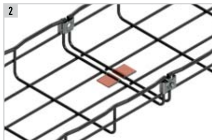
2 Position tray so that the exposed copper strips are aligned and use SWKs to join tray sections.
